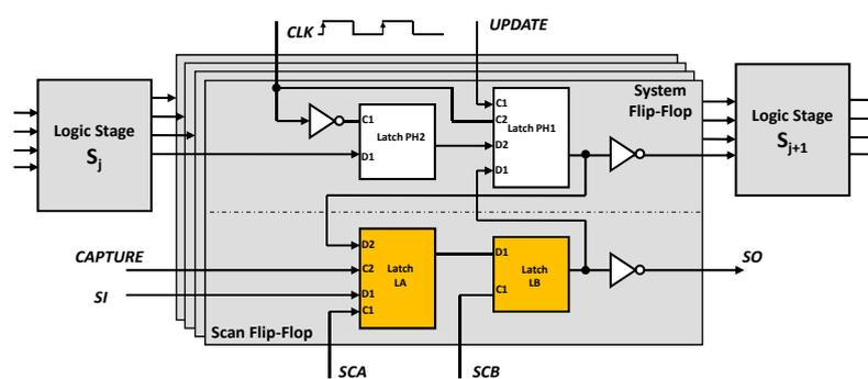
Separated System and Scan Flip-Flops
