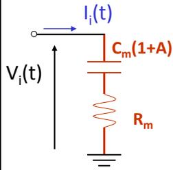
Consequently, for small  $\tau \ll$  and neglecting the independent component  $V_o^*(t)$ , the next equivalent circuit is derived, where a capacitance  $C_m(1+A)$  is in series with a resistance  $R_m$ .
