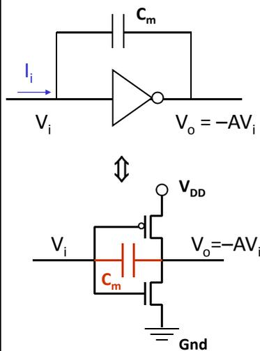
The apparent capacitance seen at the area of operation is  $C_m(1+A)$ .
