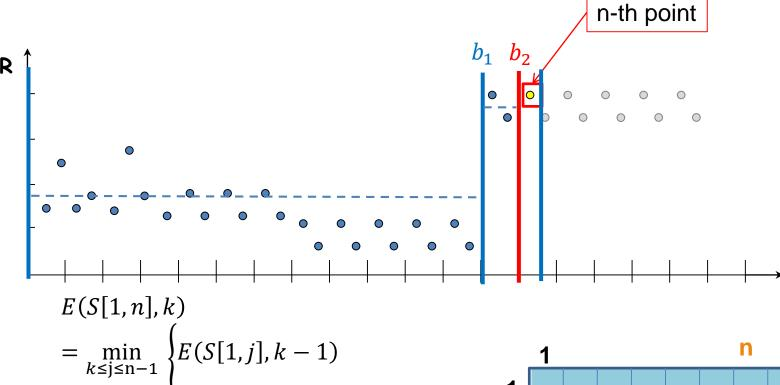
Three segnments means two boundaries  $b_1$ ,  $b_2$
