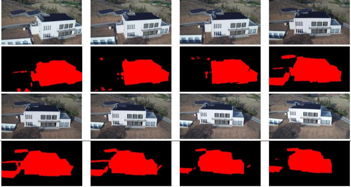
Fig. 6: Detection of main structure in each frame (2<sup>nd</sup> and 4<sup>th</sup> row) juxtaposed to original optical input frames (1<sup>st</sup> and 3<sup>rd</sup> rows). The areas marked in red correspond to the automatically detected structure.
