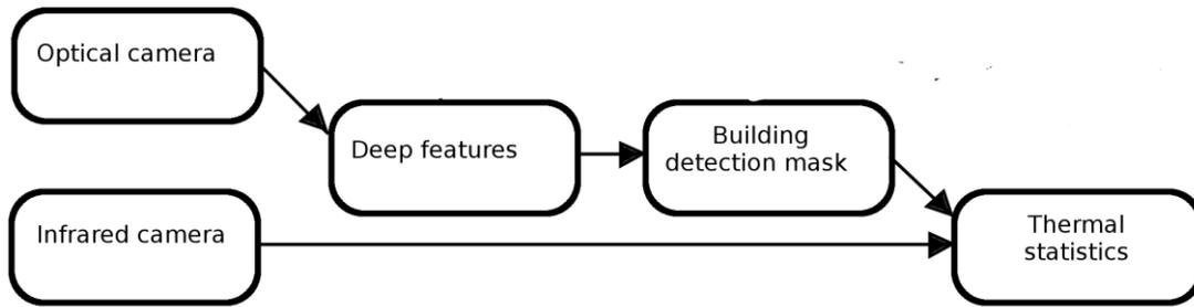
Fig. 1: Proposed image processing pipeline.
