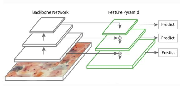
Fig. 2. Feature Pyramid Network Architecture. Bottom-up and Top-down pathway layers are connected via skip connections, and outputs are created at multiple resolutions.
