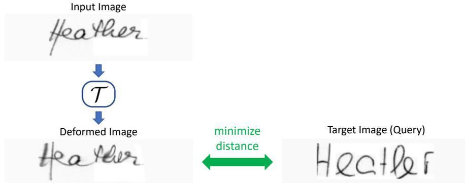
**Fig. 1.** Visualization of the paper motivation: transform an input image in such a manner that it becomes sufficiently similar to a given target image. The deformed version of the image was created by the proposed algorithm over an impractically large number of iterations (100).
