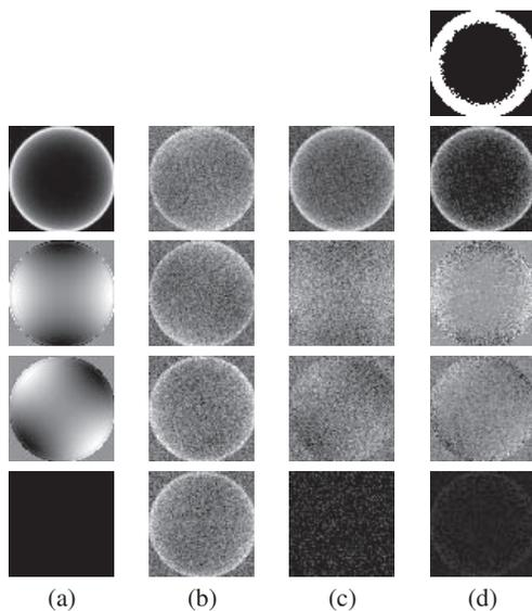
**Fig. 2.** Recovery result for simulated Stokes data under significant degradation. From left to right, each column shows the four channels of (a) the original Stokes image  $s^*$ , (b) the degraded image  $g$  (SNR of 5 dB) (c) the non-complying to Stokes constraints pseudo-inverse recovery estimate and (d) the recovered image  $\hat{s}$  obtained with our method. The corresponding segmentation of the degraded image into  $K = 2$  classes is shown at the top of the (d) column.
