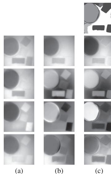
**Fig. 3.** Recovery result for real Stokes data. From left to right, each column shows the four channels of (a) the observed image  $g$  (b) the non-complying to Stokes constraints pseudo-inverse recovery estimate and (c) the recovered image  $\hat{s}$  obtained with our method. The corresponding segmentation of the observed image into  $K = 7$  classes is shown at the top of the (c) column.
