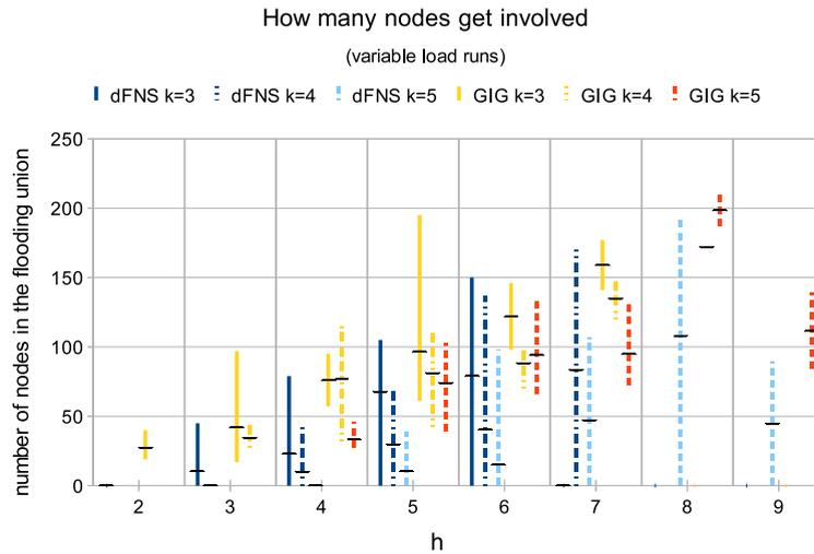
**Fig. 8.** Number of nodes involved in the flooding process (minimum, average and maximum value) using the variable load for each datanode. When lines are missing it means there were no simulation runs possible for the combination of  $k$  and  $h$  values.
