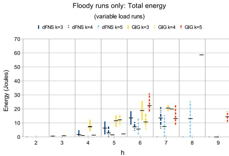
**Fig. 13.** Total energy consumed (minimum, average and maximum value) only for simulation runs that needed to use flooding in order to find the *Fermat* node. When lines are missing it means there were no simulation runs possible for the combination of  $k$  and  $h$  values.
