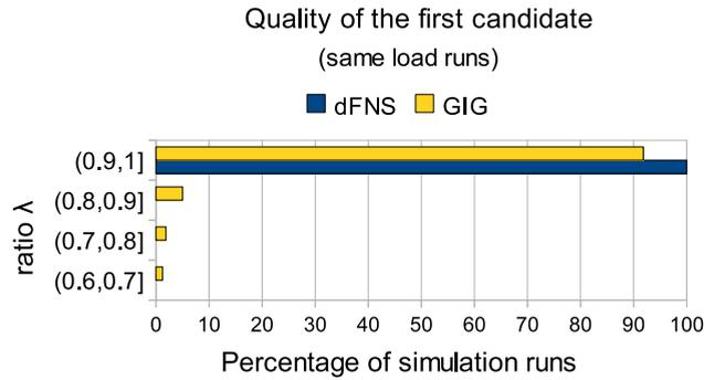
**Fig. 10.** Quality of the first candidate node encountered while flooding (or the best of the first set). Quality is expressed by dividing the hosting cost of the actual *Fermat* node to the first candidate. The closer the ratio is to 1 the better the variable speed flooding function of the algorithm used.
