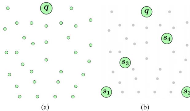
Fig. 2. Green nodes represent nodes that store data needed to answer a query  $Q$ . (a) An example of a universal query and (b) an example of a subset query. (For interpretation of the reference to color in this figure legend, the reader is referred to the web version of this article.)
