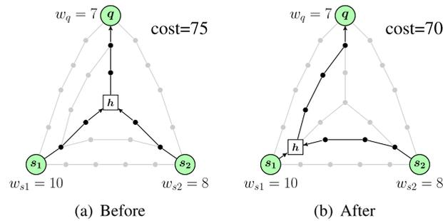
**Fig. 4.** Example of optimal operator placement: (a) Data flow during query execution before the operator placement is optimized, and (b) data flow during query execution after the operator placement is optimized. The *Fermat* node is an *external* node. The cost represents the cost of our objective function, not the actual communication cost. (For interpretation of the colors in this figure, the reader is referred to the web version of this article.)
