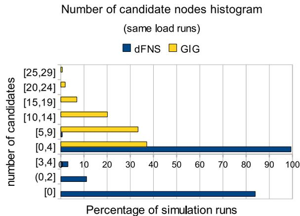
**Fig. 9.** Number of candidate nodes that report to the leader node. The less candidates the less communication needed. Beneath the x-axis the group  $[0, 4]$  is divided into more detailed groups to show the distribution for  $dFNS$ .
