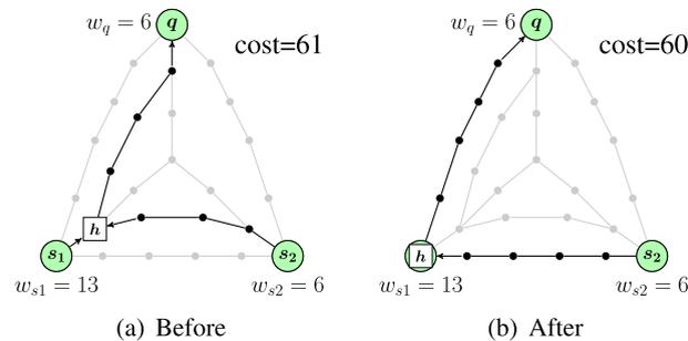
**Fig. 5.** Example of optimal operator placement: (a) Data flow during query execution before the operator placement is optimized, and (b) data flow during query execution after the operator placement is optimized. The *Fermat* node is a *datanode*. The cost represents the cost of our objective function, not the actual communication cost.
