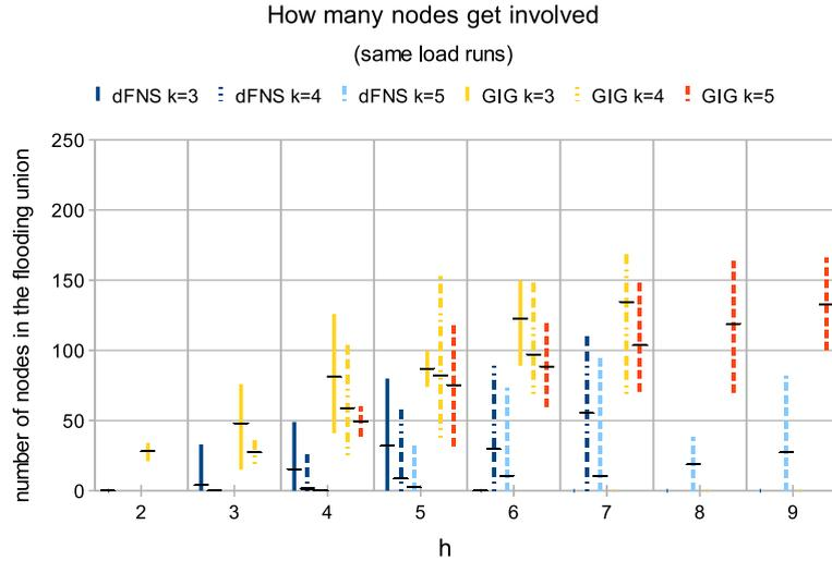
Fig. 7. Number of nodes involved in the flooding process (minimum, average and maximum value) using the same load for each datanode. When lines are missing it means there were no simulation runs possible for the combination of  $k$  and  $h$  values.
