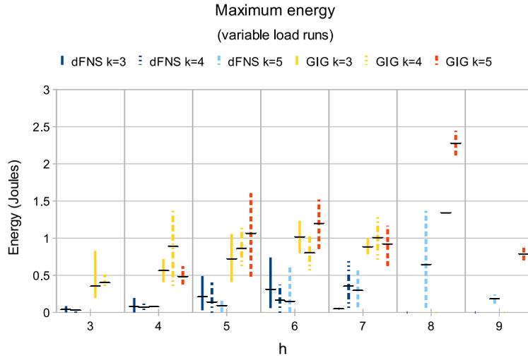
**Fig. 12.** The maximum energy consumed by a single node (minimum, average and maximum value). When lines are missing it means there were no simulation runs possible for the combination of  $k$  and  $h$  values.
