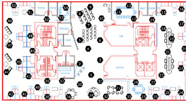
**Fig. 3.** An application example: Office building wireless sensor setup for monitoring Indoor Environmental Quality in respect to energy consumed by the building.
