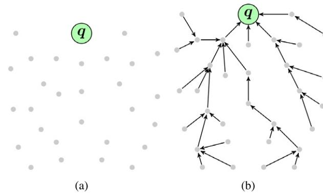
Fig. 1. (a) A wireless sensor network with a querying node and (b) a possible Query Routing Tree.
