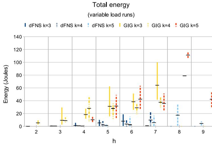
**Fig. 11.** Total energy consumed (minimum, average and maximum value). When lines are missing it means there were no simulation runs possible for the combination of  $k$  and  $h$  values.
