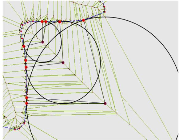
Figure 7: The largest empty circle for the farthest voronoi vertex is used in each step to identify additional feature points and update the curve.
