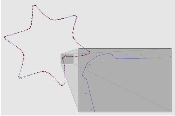
Figure 6: The convex hull method identifies internal and external slice points alternatively as feature points. If this affects the curve significantly, we may have to overcome the switching effect.
