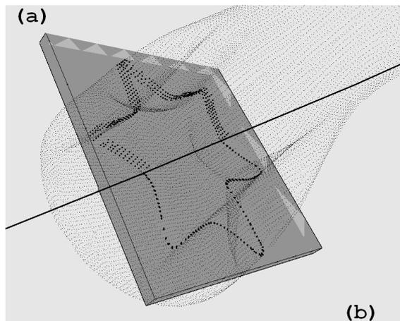
Figure 2: (a) A slice of the cloud is highlighted. (b) The points of the slice are projected on a plane parallel to the slice.
