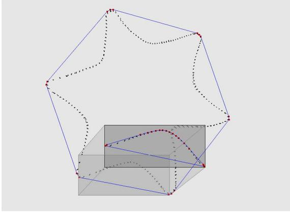
Figure 3: The points in the highlighted region are isolated and the convex hull of these points is computed to identify the next set of feature points for the curve.
