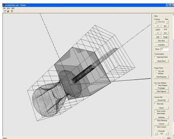
Figure 1: A point cloud can be sliced in any desired direction. Slice thickness is determined adaptively.
