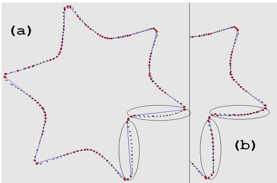
Figure 4: (a) First step of the Convex Hull Method. There are still some regions where the curve doesn't fit the points accurately. (b) Second Step of the Convex Hull Method. The curve now describes the slice points more accurately.
