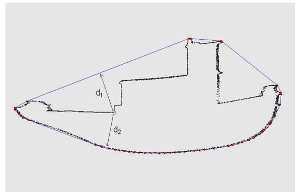
Figure 5: The points in the highlighted area are located closer to a region other than the one they should be assigned to ( $d_2 < d_1$ ). We use the information of their neighboring points to assign them to the correct region.
