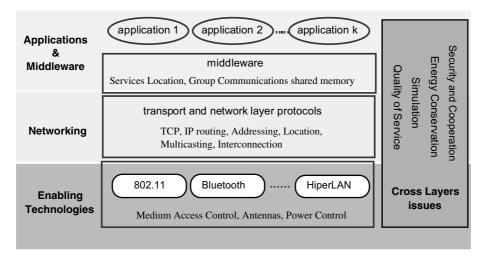
Fig. 2. A simple MANET architecture.
