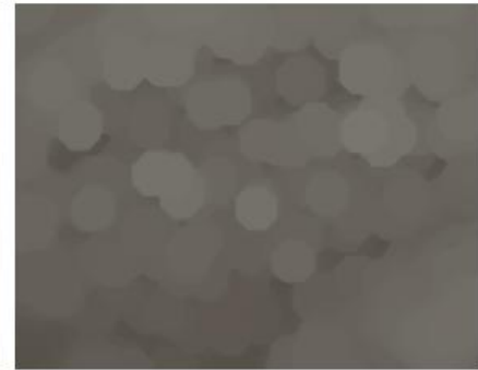
Opening by SE of radius 30 Large dowels disappeared.
