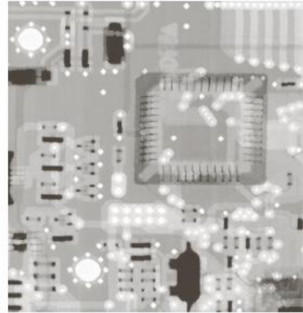
Dilation by a flat disk SE of radius 2: Lighter background, small dark dots reduced, light features grew.
