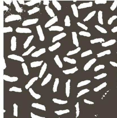
Thresholded image (Otsu's method)
