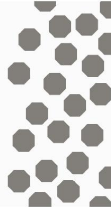
Closing with a SE of radius 30 (small blobs are removed)
