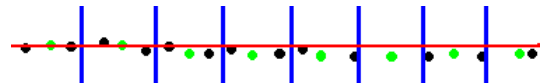
Fig. 2. An example of the sampling process. The black points represent the original set of points, while the red line is their summary computed by DSaM [9]. The vertical blue lines depict the limits of the histogram bins. The green points are those selected to represent the sampled set because they are closer to the mean value of the bin. The figure is better seen in color.
