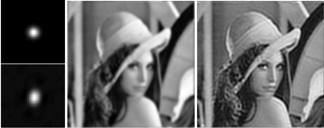
Figure 3: Gaussian PSF with small support. Images (left to right) of the true PSF that was used to generate the degraded image (top), the estimated PSF (bottom), the observed image and the estimated image.
