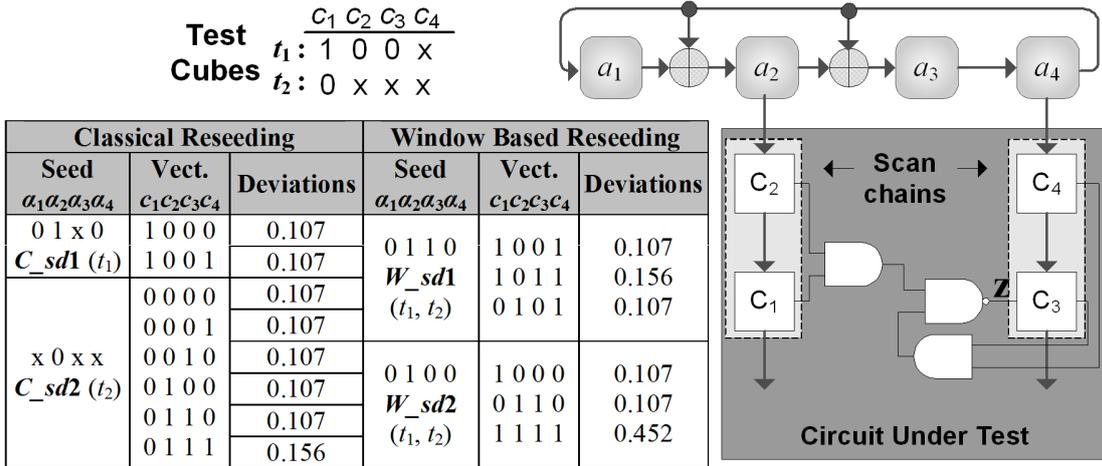
Figure 2: Example of classical and window-based LFSR reseeding
