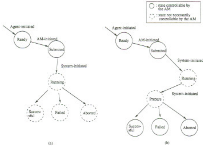
Figure 1: Controllable states for basic methods, when: (a) there is no prepare-to-commit state, (b) there is a prepare-to-commit state
