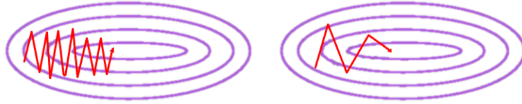
Figure 2.5: Left: Standard SGD. It is clear that SGD oscillates highly across the ravines. Right: SGD with momentum. The oscillations across the steep direction are dampened and momentum moves faster towards the relevant direction. Figure reproduced from [2]
