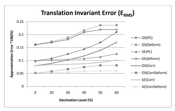
Figure 6. 20: Balloon approximation error  $E_{RMS}$  progression due to decimation.
