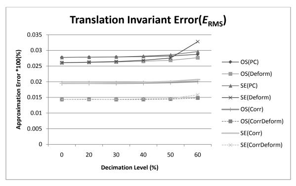
Figure 6. 16: Camel collapse approximation error  $E_{RMS}$  progression due to decimation.
