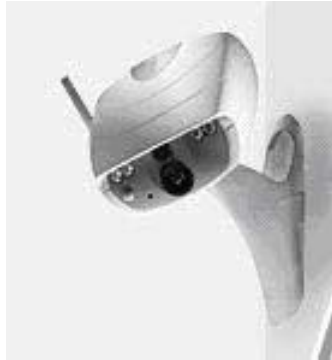
Figure 2.2: Nokia Observation Camera sending MMS or e-mail messages with image and temperature data.
