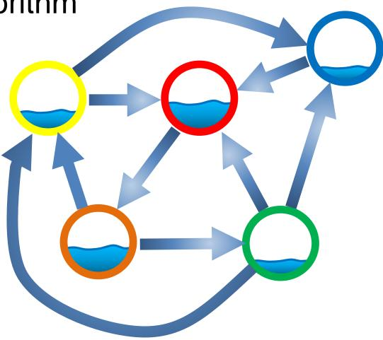
The amount of liquid in each node determines the importance of the node.
