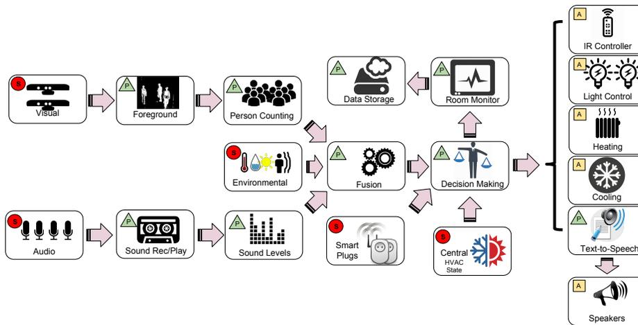
Figure 1: High-level architecture of the smart room application.
