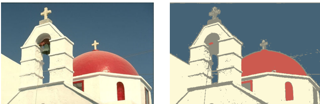
Figure 3. Natural image segmentation using Lab features for \epsilon = 5 , K = 7 initial number of segments. The algorithm converged to four segments.
