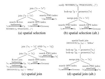
Figure 3: Query plans in the basic extension
