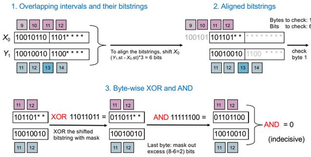
**Figure 5: Intervals [9, 12] and [11, 14] of our two example polygons overlap but are not aligned. Byte truncation and bit shifting (if necessary) align their bitstrings before performing the bitwise operation(s)**
