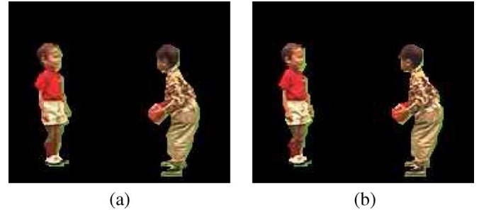
Fig. 2. Frame no. 0 (“Children” sequence). (a) SA-DCT based texture coding, Th = 600 , Bias = 0.5 , QP = 4 , R_{total} = 21356 bits, D_{texture}^{YUV} = 10.14 . (b) SA-DWT based texture coding, Th = 600 , Bias = 0.5 , Decoding rate = 21848 bits, D_{texture}^{YUV} = 2.63 .
