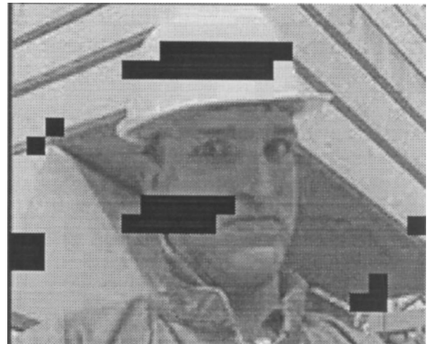
Fig. 14. Missing block location of 1st frame of foreman sequences (intra frame).
