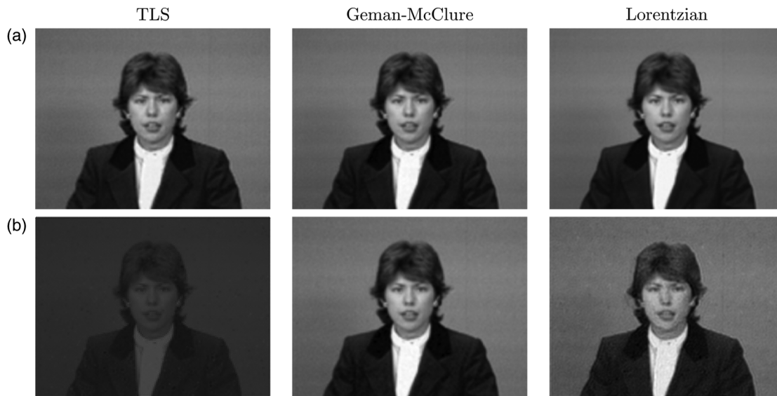
Fig. 4 Reconstructed high-resolution images for 20 frames of the Claire sequence, with speckle noise at 1%. (a) Robust parameters \varepsilon_k and \alpha_k(\mathbf{z}) and (b) no robust parameters.
