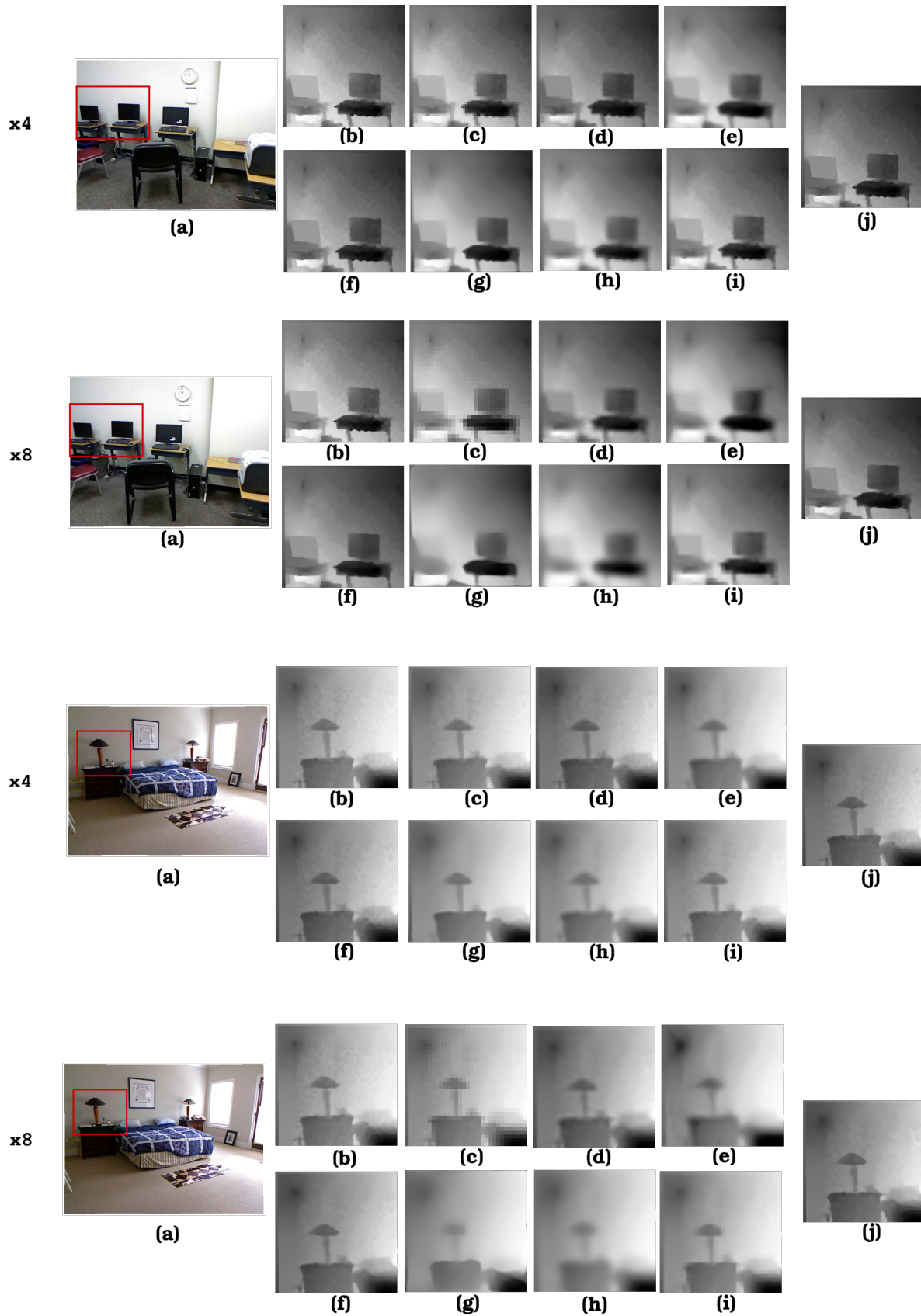
Figure 4. Depth map SR results for upsampling factors \times 4 and \times 8 . The reconstructed depth maps obtained with our method in (i) are compared with (d) bicubic interpolation, (e) BM3D-ADMM [35], (f) the method of de Lutio et al. [15], (g) DnCNN-ADMM [45], (h) TV-ADMM [34], and (j) DAGF [46]. We also present (a) the HR color image, (b) the ground truth, and (c) the downsampled depth maps.
