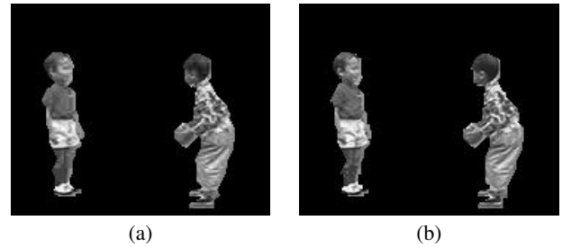
Fig. 2: Frame no. 80 (“Children” sequence),(a) SA-DCT based texture coding, Th = 600 , Bias = 0.5 , QP = 4 , R_{total} = 21356 bits, D_{texture}^{YUV} = 10.14 , (b) SA-DWT based texture coding, Th = 600 , Bias = 0.5 , Decoding rate = 21848 bits, D_{texture}^{YUV} = 2.63 .
