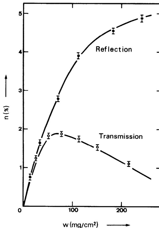
FIG. 7. Calculated and experimental x-ray luminescence efficiency vs screen's thickness for ZnCdS:Ag screens in transmission and in reflection mode observation. Dots: experimental data; lines: theoretical results.
