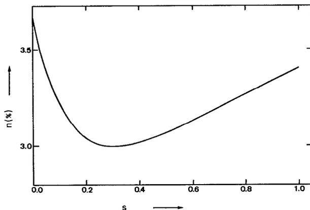
FIG. 6. Calculated x-ray luminescence efficiency (peak values) of a phosphor screen vs the light-scattering coefficient.
