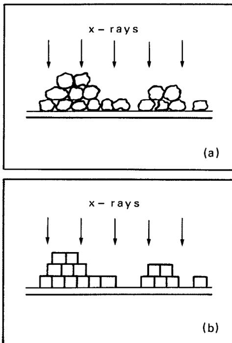
FIG. 1. Cross sections of a phosphor screen: (a) real structure and (b) modeled structure.
