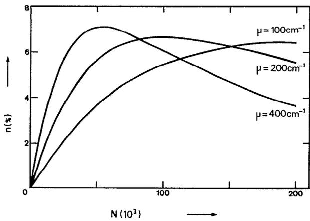
FIG. 3. Calculated x-ray luminescence efficiency vs screen's thickness (number of phosphor grains on the screen's substrate) for three different x-ray-absorption coefficients.
