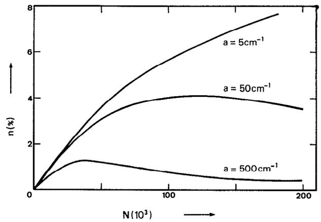
FIG. 4. Calculated x-ray luminescence efficiency vs screen's thickness (number of phosphor grains on the screen's substrate) for three different light-absorption coefficients.
