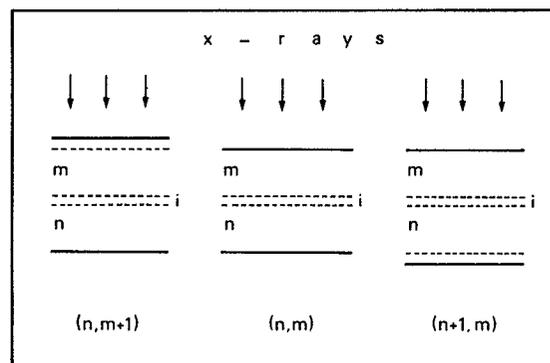
FIG. 2. Cross section of a part of a phosphor screen (for the development of the recursion relation for the light fluxes emitted from it).
