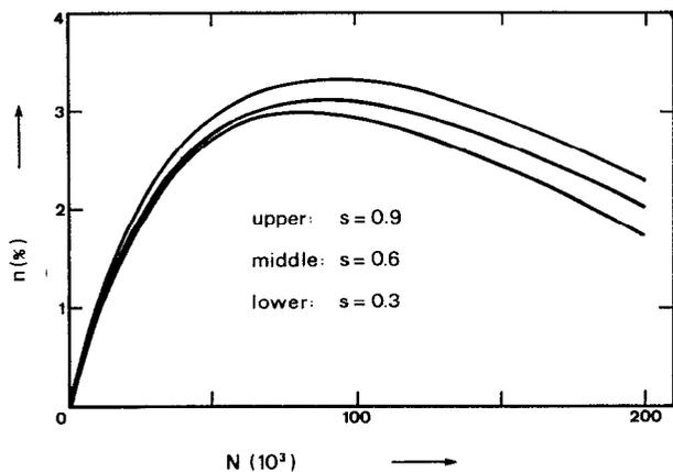
FIG. 5. Calculated x-ray luminescence efficiency vs screen's thickness (number of phosphor grains on the screen's substrate) for three different light-scattering coefficients.
