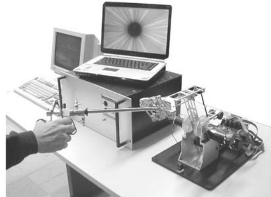
Fig. 2. Haptic mechanism, part of the training urological simulator during a test session.
