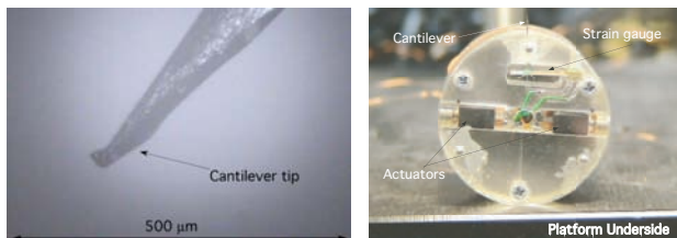
Fig. 13: Cantilever: a. Microscope view b. Strain gauge installation
