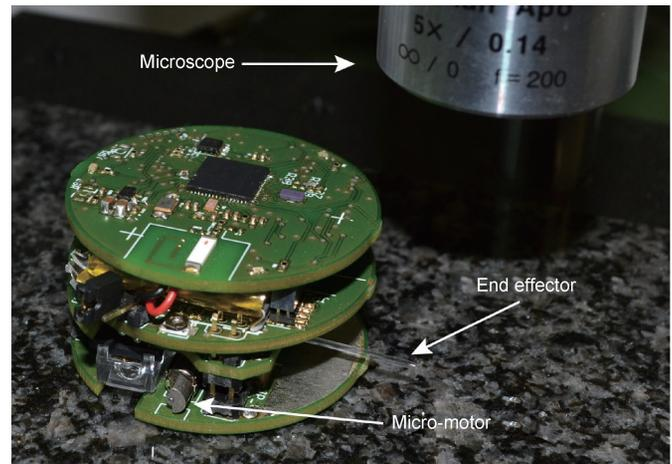
Figure 7. Microrobot under the microscope.
