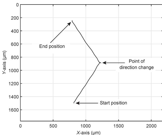
Figure 12. End-effector path using the open-loop approach.
