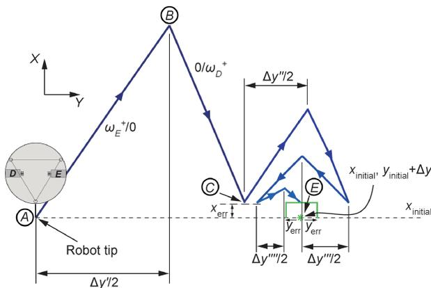
Figure 9. Schematic description of the CL2 algorithm.
