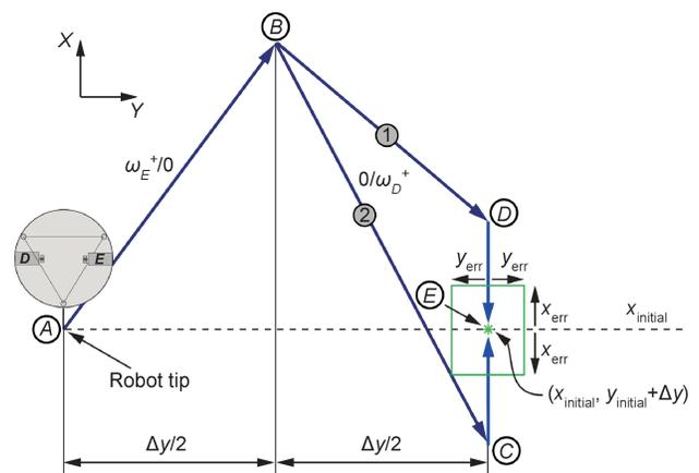
Figure 8. Schematic description of the CL1 algorithm.
