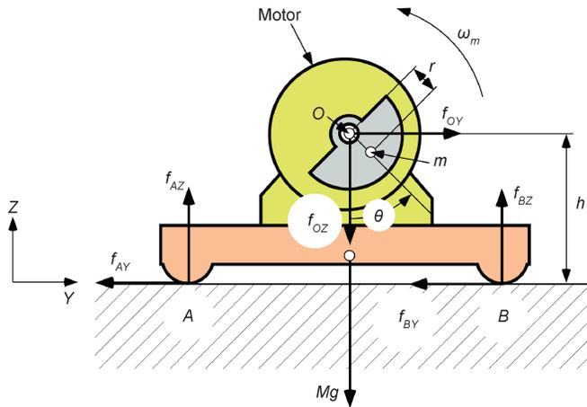
**Figure 1.** Simplified 1-DOF platform with eccentric rotating mass  $m$ . In the figure,  $m$  is pointing at the center of mass of the eccentric part, which has an offset  $r$  with respect to the axis of rotation.
