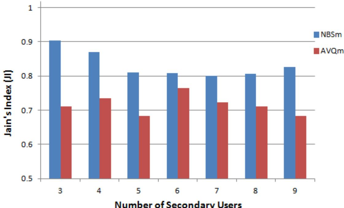
Fig.7: Average JI for different number of SU (M=4, CNR=25 dB, Multiple Video Transmission).
