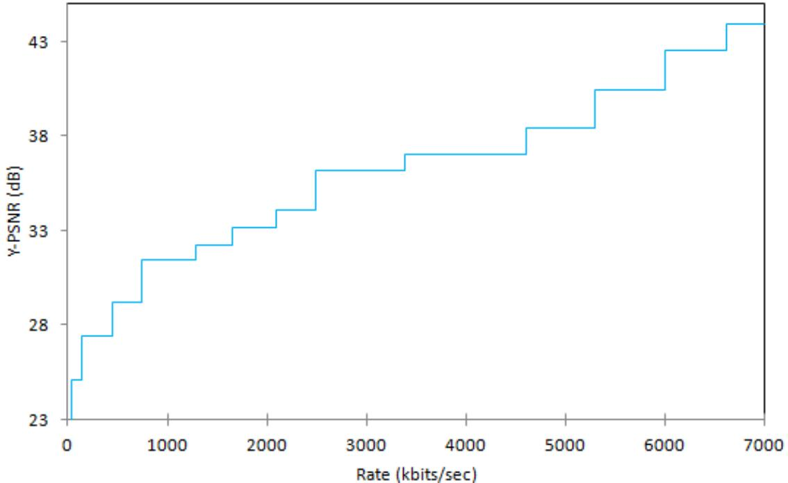
Fig.4: Quality-rate plot with MGS encoding for “Coastguard” sequence.
