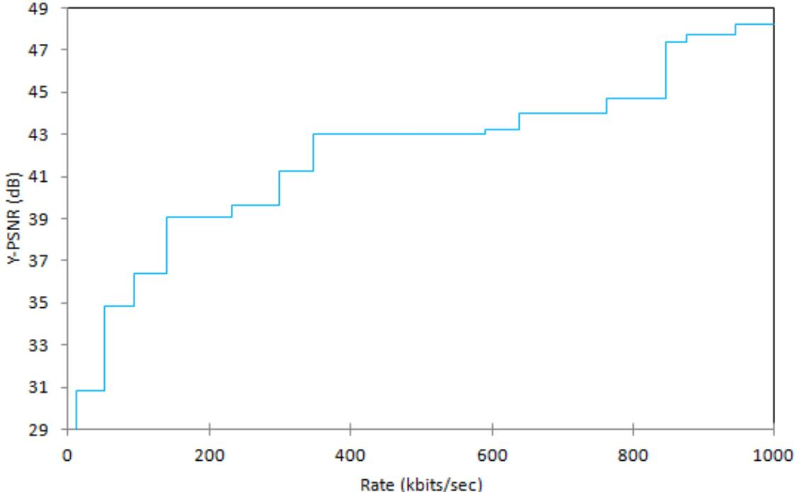
Fig.5: Quality-rate plot with MGS encoding for “Akiyo” sequence.
