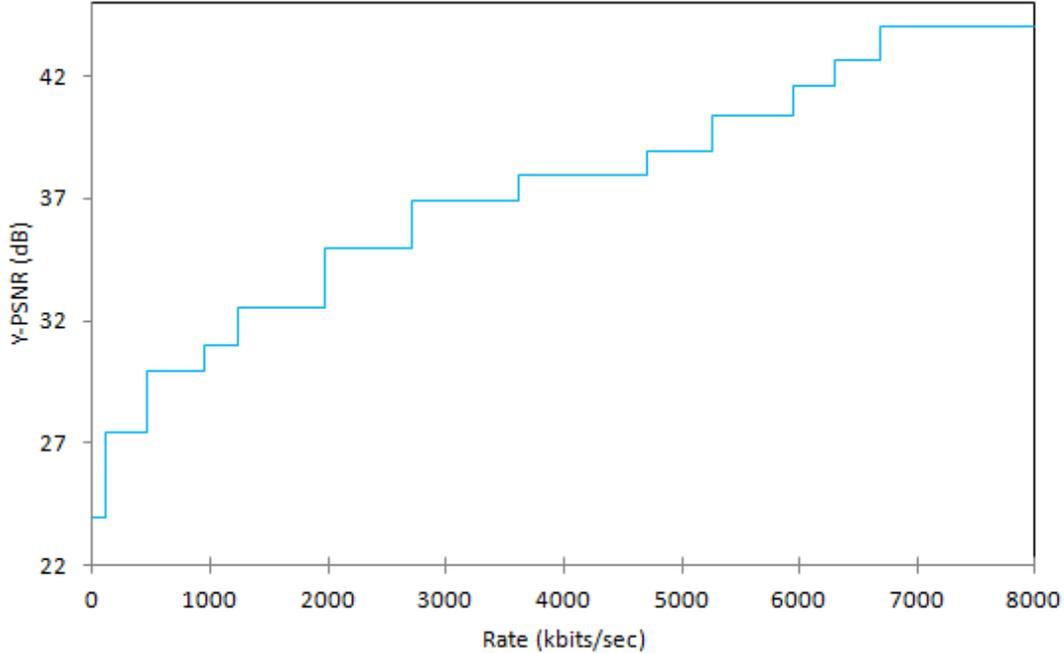
Fig.2: Quality-rate plot with MGS encoding for “Bus” sequence.
