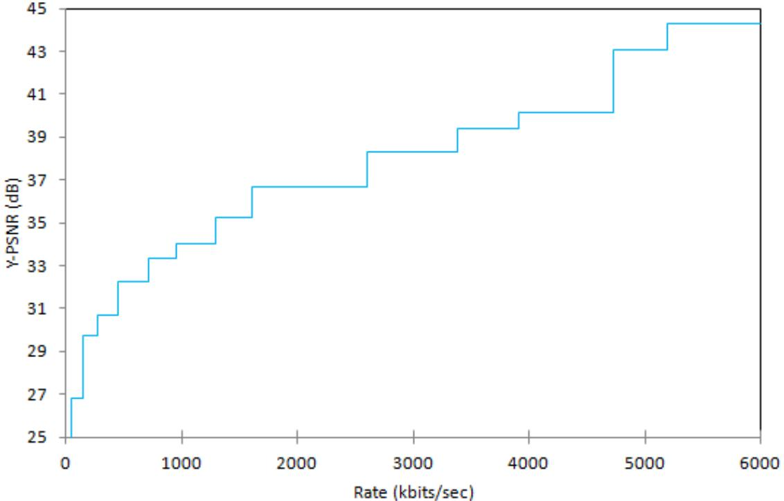
Fig.3: Quality-rate plot with MGS encoding for “Foreman” sequence.
