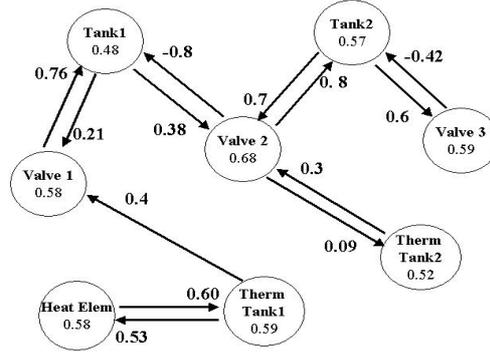
Figure 4: The FCM model for the process control problem.
