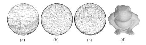
Figure 1: (a) The result of the initial mapping using the planar barycentric method, (b) the Laplacian smoothing technique, (c) the result after optimization and (d) the original frog model.
