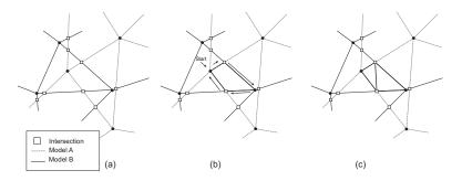
Figure 2: (a) Finding intersections in merged topology, (b) curve faces visited in clockwise manner and (c) triangulation
