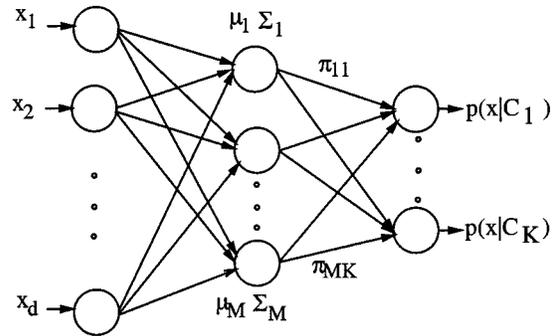
Fig. 1. The architecture of the probabilistic RBF network.
