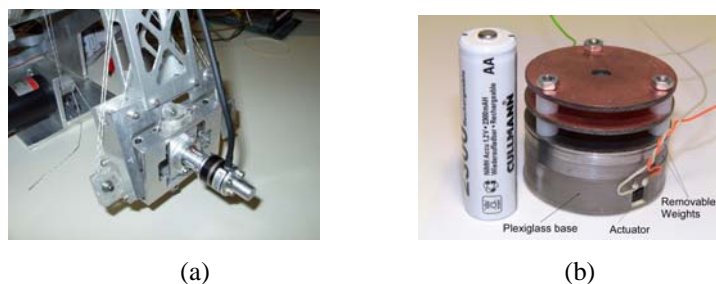
Fig 1. (a) The haptic master device. (b) The slave microrobotic platform.
